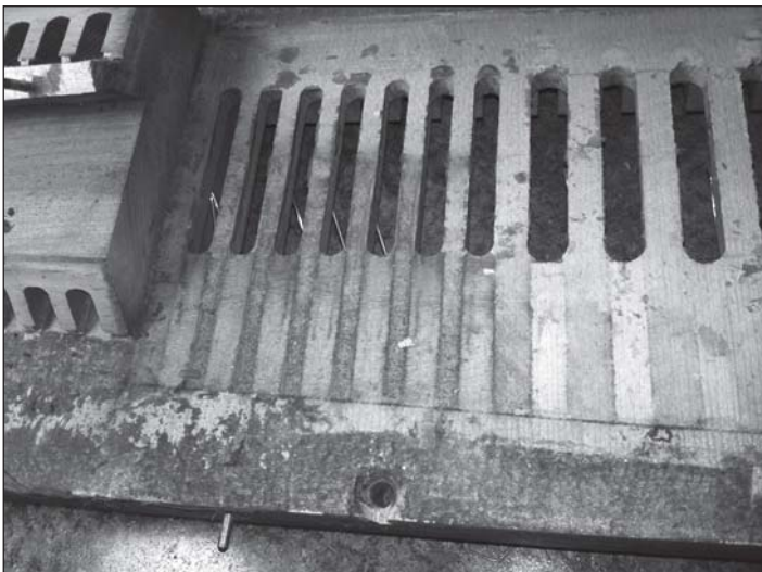
Windchest after removal of loose reed cell section. Note dark coal soot buildup in between pallet holes where the reel cell normally would have been glued down.
