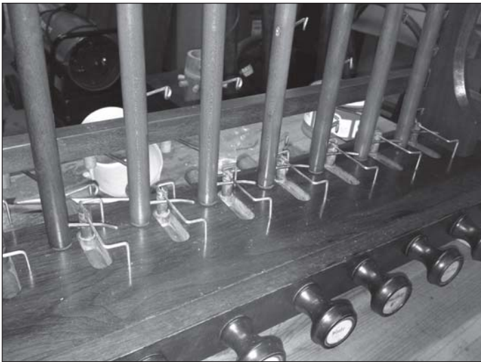
Stop action transfers to vertical windchest by rotating dowels.
