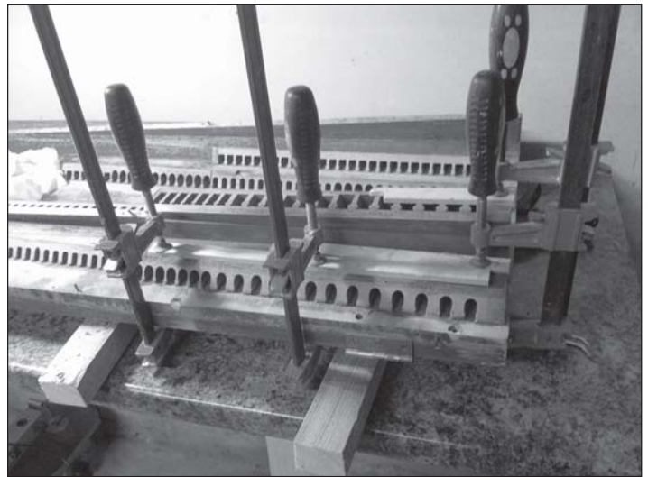
Loose reed cell section cleaned and glued back in place.
